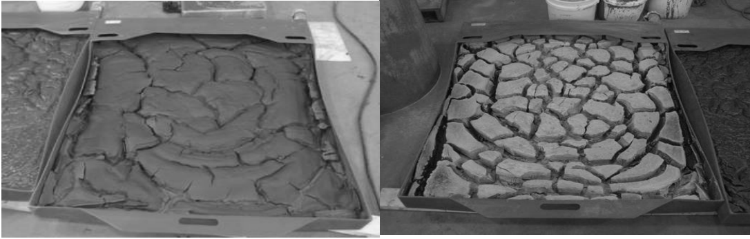
FIGURE 3. Untreated MFT (left) and a gypsum/lime treated MFT (right). Under the same conditions, the treated MFT has dried considerably faster.
